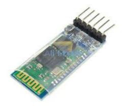
The blue tooth module must be configured to operate at 38400 baud. This can be done by using the blue tooth terminal application for the M3 or M4 processor found in the downloadable file bt\_terminal.zip.
